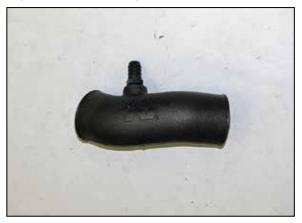
6. Install the provided crank case vent fitting into the  $K\&N^{\otimes}$  intake tube as shown.
