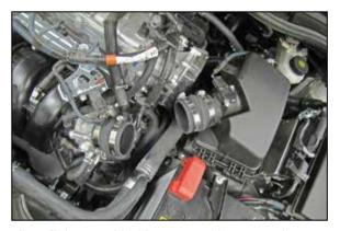
5. Install the provided hump couplers onto the throttle body and air filter housing and secure with the provided hose clamps.
